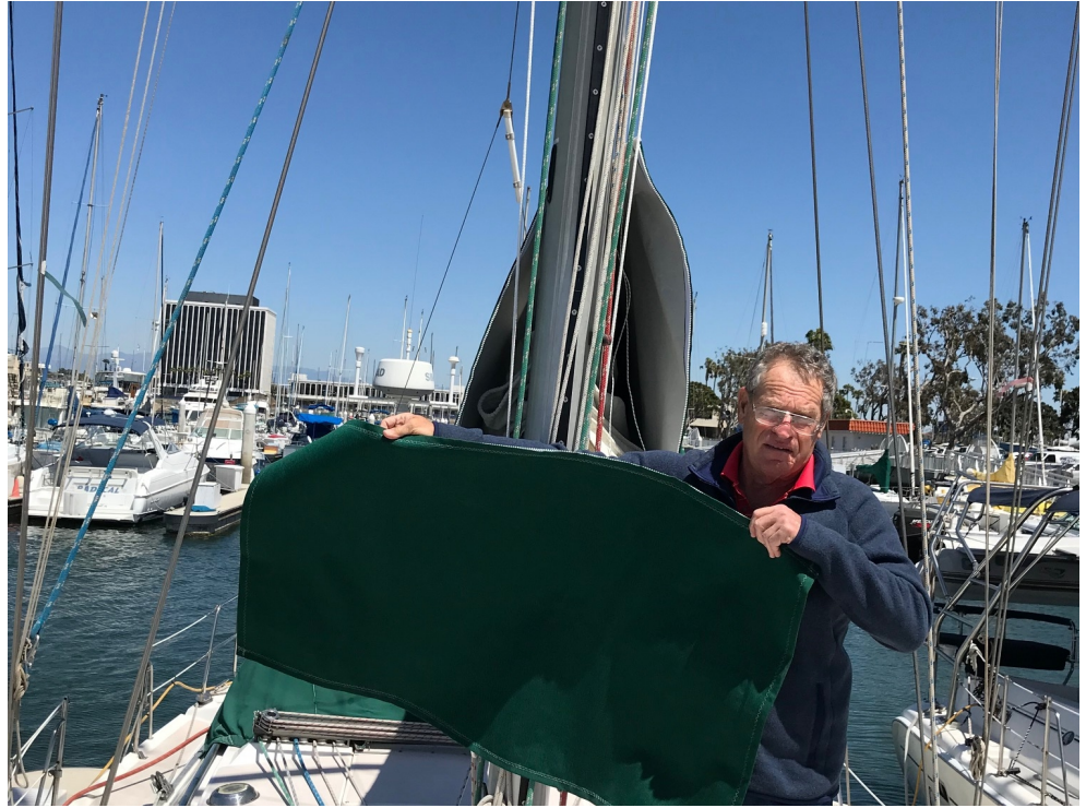
Marv Brown demonstrates how to remove the front panel, which must be stowed below
