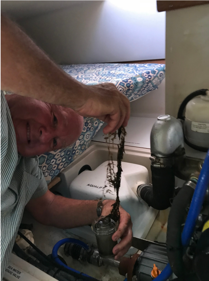
Ron Sasiela extracts a piece of slimy seaweed from Kestrel's raw water filter.
