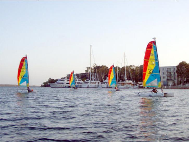
The Hobies sail down wind with one rudder up to minimize drag.
